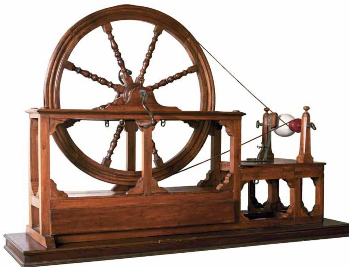
Fig. 5. Electrical machine built in Florence in the last quarter of the 18<sup>th</sup> century, Nollet type; Museo Galileo, inv. nos. 2737, 1341, 1342.
