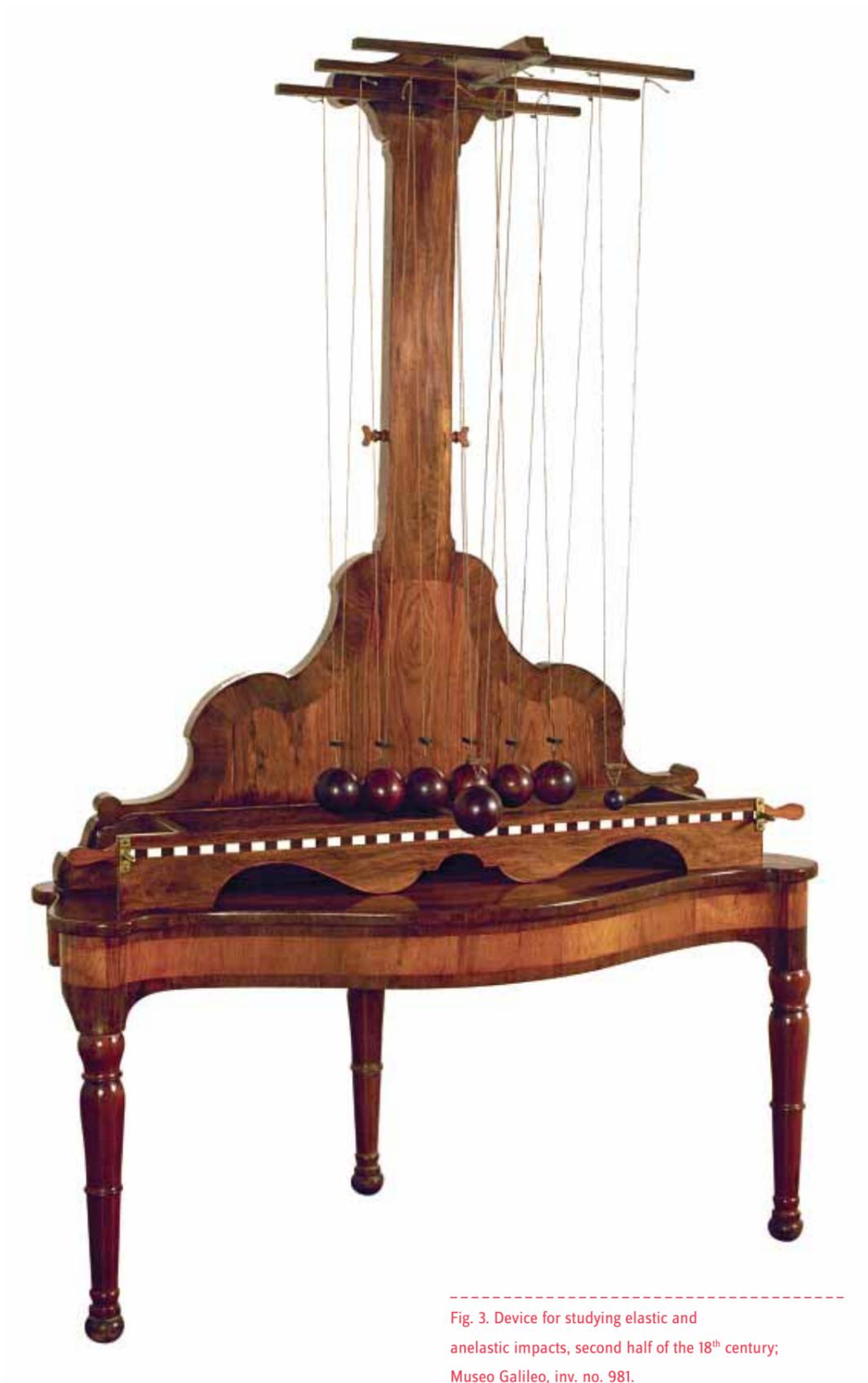
Fig. 3. Device for studying elastic and anelastic impacts, second half of the 18<sup>th</sup> century; Museo Galileo, inv. no. 981.
