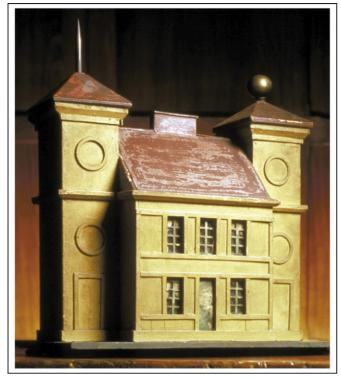
Figure 3. Thunder house with lightning rod. An operator would make a spark strike the pointed metallic conductor on top of the house, simulating lightning. If the conductor was grounded, nothing would happen, thus demonstrating the value of lightning rods. However, if the conductor were was not grounded, the spark would ignite some gunpowder placed inside the house, resulting in a dramatic explosion. Courtesy of the Bakken Library and Museum for Electricity in Life.
